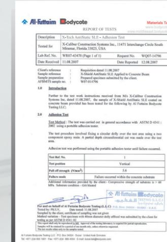
ASTM D4541 Adhesion Test
